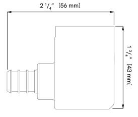
This inlet replaces the default hydrant inlet with a 1/2'' PEX Crimp connection. Quickly and reliably connect your Aquor hydrant to 1/2'' PEX tubing for an easier installation. The elbow inlet shortens the overall length of the hydrant by 1/2''.
