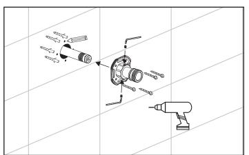
[Step 1] Apply a generous amount of PTFE (plumber's) tape to end of end of nipple (4).
