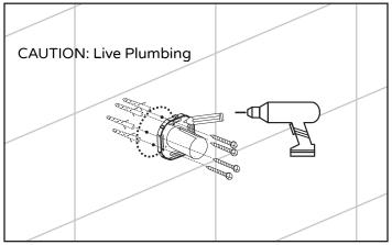
Place lower mount plate (26) on marked location and mark holes for drill option.
