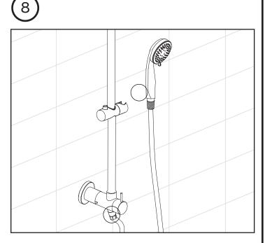
Insert washer (22) into the hex end of the hand shower hose (23). Attach hose to hand shower (20) outlet located on the bottom of the diverter (29). Insert washer (22) into the tapered end of the hand shower hose (23) and attach the hand shower (20). Place the tapered end of the hose into the hand shower holder (19).
