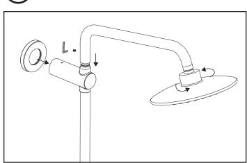
Remove plastic cover and slide Shower Arm (15) onto Top-T (30). Connect Shower Head (17). Slide in escutcheon (11). Screw shower head (17) onto shower arm (15). Allen wrench with 2 size ends
