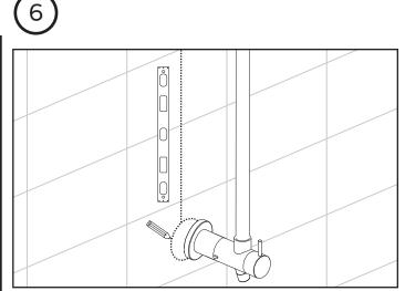
Use level to assure shower pipe is straight and mark lower diverter (29) mount location.
