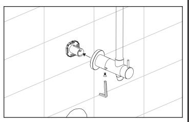
Slide bottom diverter (29) and cover mount (24) onto lower mount plate (26) and secure with set screw (25).
