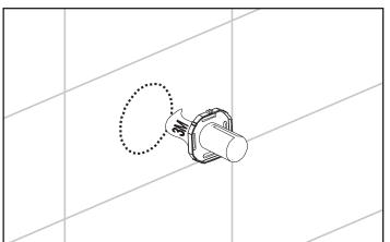
Hold for about 30 seconds to dry. Tape will be fully cured after 24 hours.
