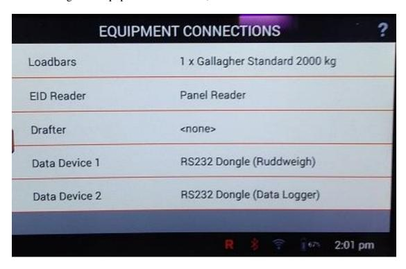
XI. Data Device 2 is for sending 'EID', so ensure "type" is "Data Logger" and the "send" setting is "on animal release" select 'save'. NOTE: It is important that the unit set to "on animal release", otherwise if the weight is locked, the EID will NOT be sent
