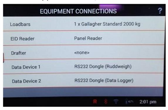
IX. Data Device 1 is for sending **weight**, so ensure "type" is "Ruddweigh" and select 'save'.
