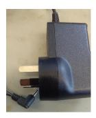
In our setup we are using the external Bluetooth dongles that are used with W810 etc. These devices require power, and we will be providing power from an external 7.5 v power supply, therefore the mode must be changed to 'Adapter' via the switch on the side of the dongle.
