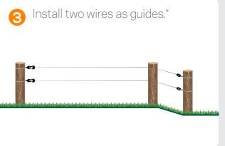
Install the line posts 7-10m apart. Install insulators\* and fit remaining wires.
