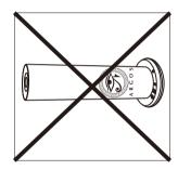
After installation, please keep the machine vertical. Tilted or angled may cause oil overflow, which will contaminated equipment circuit, affecting the normal use and unnecessary waste.
