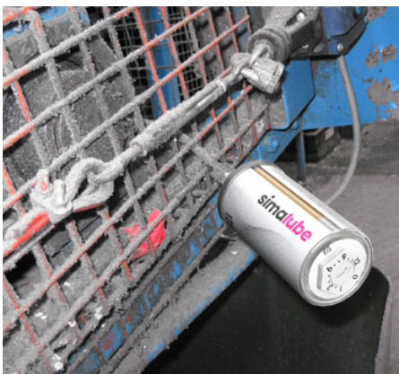
The externally installed simalube prevents dirt from entering the lubrication point.
