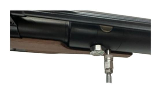
Insert the fill probe into the air filling hole.
