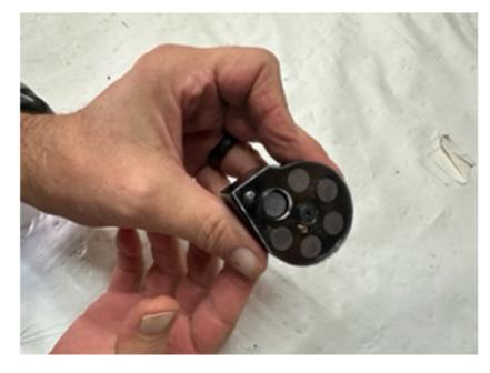
Load slugs by pushing the transparent cover counter clockwise until the cover stops. Keep the cover open in the end position.
