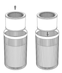
3. Reattach the filter cover and twist clockwise screw nut to lock.
