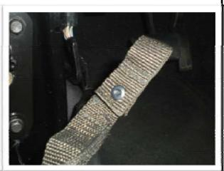
9. Plug the electrical connection back into place & then reattach the lengthen fabric door strap. Attach the factory mirror. Check to make sure that the door runs smoothly & make sure that nothing is binding. If you feel binding in the door **STOP** moving the door as it will damage the part. Check to make sure that everything is aligned. There is room to adjust the part if needed.
