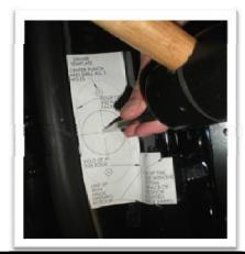
5. Now insert the Smart Door Check Strap into the newly drilled 1-3/4" hole & then attach the arm bracket onto the screw posts on the newly installed hinge plate bracket. Secure arm bracket into position using the supplied 10mm nuts & washers. Now make sure that the upper & lower center punch marks are lined up horizontally before drilling the holes. Remove the part & then drill the upper & lower holes using
