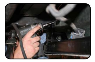
Remove sway bar links at the axle using 18
