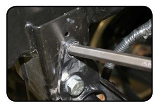
12. Install the alignment spacer onto the drivers side of the shaft and leave loose.
