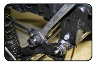
Tighten the sway bar arm pinch bolts using a 9/16 socket and wrench. Torque to 50 Ft-lbs
