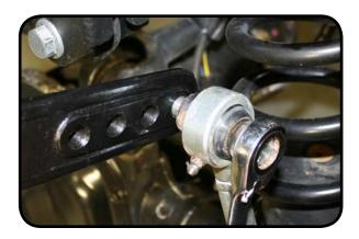
22. Install the bottom sway bar link at the inside of the axle tab using the factory hardware and torque to 75 Ft-lbs.
