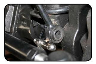
3. Remove the bolts from the sway bar mount using a 16mm socket. Make sure the sway bar is supported while removing the bolts from frame. (If Rubicon, disconnect the wire harness at the sway bar prior to removing mounting bolts)
