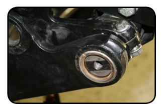
17. Install the end cap using 9/16" socket and blue thread locker. Make sure that the slot key engages with the torsion shaft. Torque both end caps to 20 Ft-lbs.
