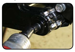
18. Install the locking knob into the arm using a 1 1/2" open wrench and blue thread locker.
