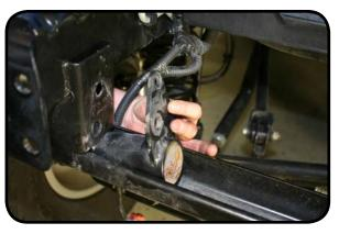
7. Install the 9/16" x 1 1/2" bolt into the outside welded nut using a flat washer and lock washer.
