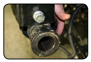
10. Grease the inside of the bushings and install the main shaft.
