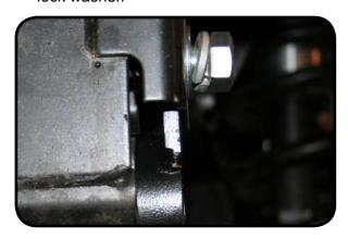
8. Install the two inside lower bolts using the supplied 9/16"x1/2" bolts and lock washers. Use an 7/8" open end wrench and tape, hold the nut on the wrench. Start the nut and leave loose.
