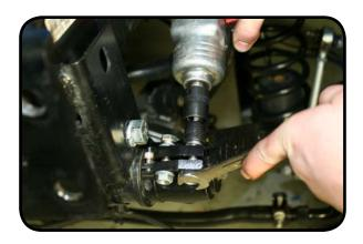
20. Tighten the alignment spacer bolt using 3/16" allen.
