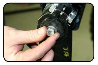
15. Install the locking arm on the shaft of the passenger side.
