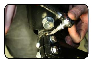
21. Install the top sway bar links on the outside of the sway bar arm using the supplied hardware and 3/4" socket or wrench. Torque to 75 Ft-lbs, use blue thread locker.
