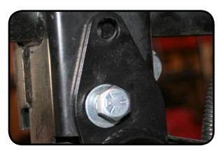
9. Install the bushings into the mounts on the frame.
