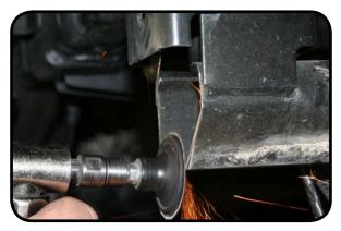
5. For 2011 measure 4 5/8" from the top of the cross member down. Use a square to scribe the line. Cut and remove the section the covers the cross member. Cut the welds and grind smooth.
