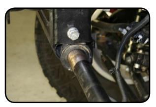
11. Tighten the bushing mount bolts. Use a alignment tool to keep the upper hole aligned. Then install the upper mount bolt and Torque bolts to 55 Ft-lbs.
