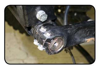
14. Install the end cap so that the slot key engages with the torsion shaft and leave loose. Use blue thread locker th prevent the bolt from comming loose.
