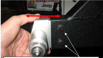
You can loosen the two bolts on the handle block and move slightly inward or outward.
