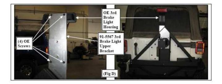
Step 9: Reattach the third brake light wiring harness you previously removed.
