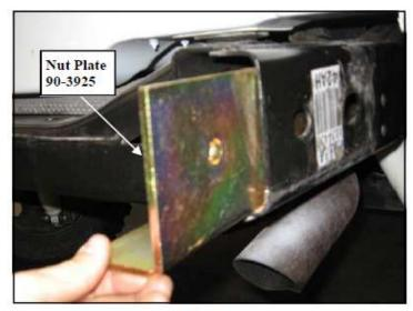
Step 3: Insert nut plate (90-3925) into the inside of the rear frame rails. (Fig B)
