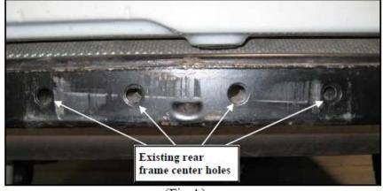
Step 2: Drill out the (4) holes in the center of the frame to 1/2". (Fig A)
