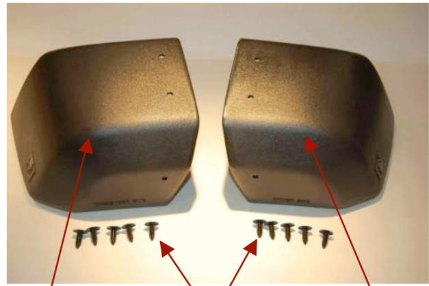
**Passenger Side 10 Plastic Pin Plugs Driver Side**
