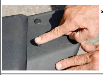
5) With the Holes aligned - Install the Black Plastic Pin Plugs pushing through the Bumper Cap into the holes in the bumper. You are now complete and the Bumper Cap is Installed.
