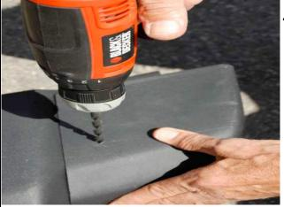
4) Using a 1/4" Drill Bit - Drill the installation holes using the Five (5) pre-drilled holes in the Bumper Cap as a guide
