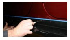
4. Drill a 25/64 hole at each mark to prepare for installation of the nut inserts. Install the nut inserts along the body using an appropriate insert tool. Note: avoid drilling into the wiring harness along the bottom of the door when drilling all the holes.
