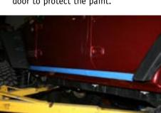
3. Hold the new rock slider up in place and mark all the holes on the tape using a black marker.
