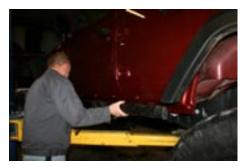
2. Put tape along the body under the door to protect the paint.
