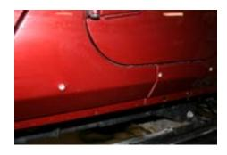
5. Put the rubber seal along the top edge of the rock slider and cut to length. Install the slider along the body with the stainless button head bolts.
