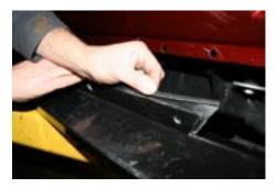
With the body side bolts installed, mark and drill up through the bottom of the rock slider and install the long through bolts.
