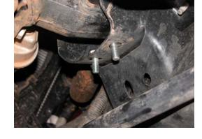
**Step 3:** Install the passenger side-mounting bracket using the bolts just inserted into the motor mount. The mounting tab faces the rear of the vehicle. It is shown with the strut rod attached in the photo to the left. Leave these bolts loose for now.
