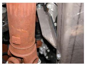
**Step 10:** Install the driver's side strut rod as shown at left. Make sure to place the strut rod within the skid plate as shown.
