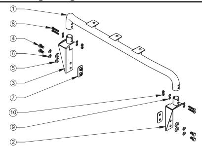
07-09 JK: Locate the two frame mounting holes behind the bumper on the left side of the vehicle. Slide the Nut Plate behind the two holes. Use the M12 Hex Bolts, Lock Washers and M12 Flat Washers to secure the Left Side Bracket to the frame as shown. Do not fully tighten the bolts at this time. Repeat for right side.
