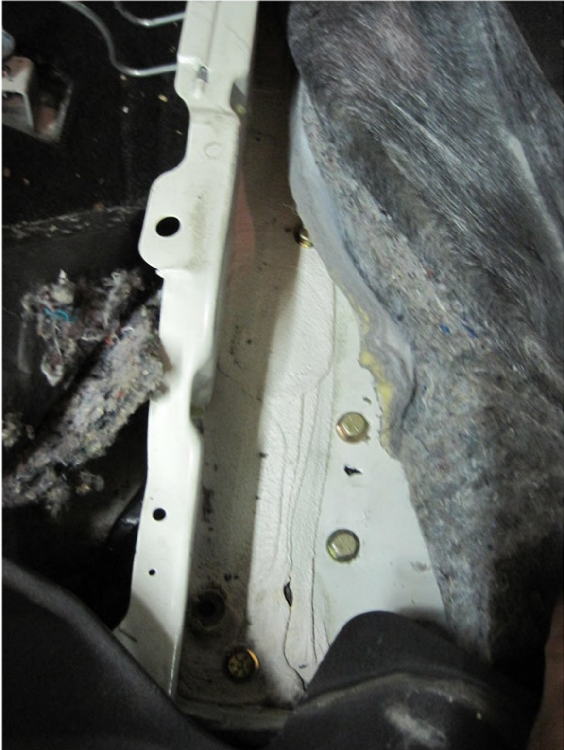
Top view of spring hanger bolts, looking down under the rear seat.
