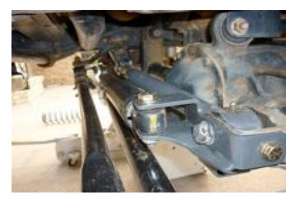
10. Position the tie rod clamp so you have full steering and full travel of the steering stabilizer. Make sure that tie rod clamp is rotated forward enough so the steering stabilizer does not move back into the diff cover when you turn right. Torque the socket head bolts to 20 ft-lbs(27 N-m) and ½" bolt to 75 ft-lbs (100 N-m) on the PPM-8003 tie rod clamp.
