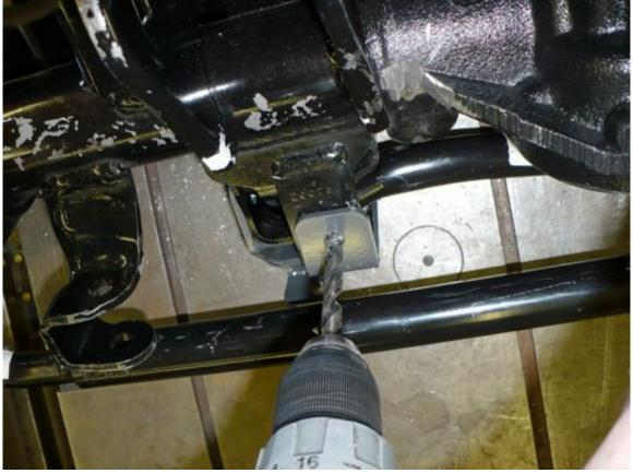
6. Install the two additional 3/8 bolts to the factory track bar bracket. Use a washer under both the head of the washer and under the head of the nut. Torque these bolts to 40 ft-lbs (54 N-m)
