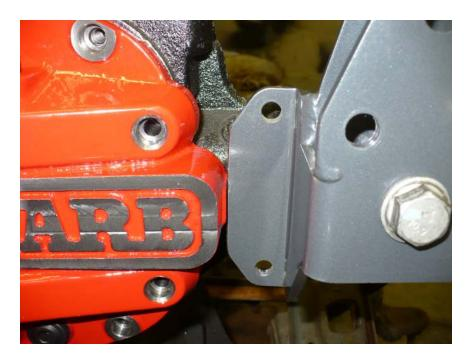
4. Position the new PPM-8091 track bar bracket over the stock track bar bracket as shown below. Secure the bracket to the sway bar tab using the supplied 1/2 x 3" bolt and spacer. There are 3 cylindrical spacers included with this kit, use one of the longer 1.5" (38mm) ones for this step. Use a washer under the head of the bolt and under the toplock nut. Do not tighten any of the track bar bracket hardware until all of the hardware is installed.
