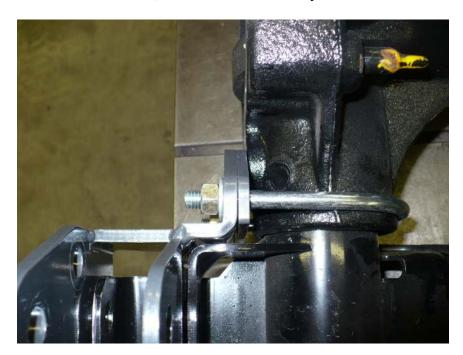
7. If you have a Rubicon with a Dana 44, you will have to grind the bottom web slightly to clear the u-bolt. Do not use the shim. Install the u-bolt over the axle housing and through the track bar relocation bracket, use a flat washer and nylock nut to secure the u-bolt.
