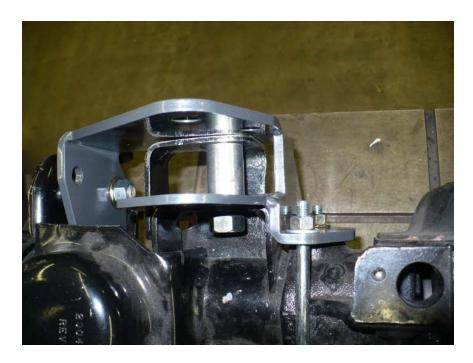
6. If you have a Dana 30, use the supplied shim between the housing and the track bar relocation bracket. Install the u-bolt over the diff housing and through the track bar relocation bracket, use a flat washer and nylock nut to secure the u-bolt.
