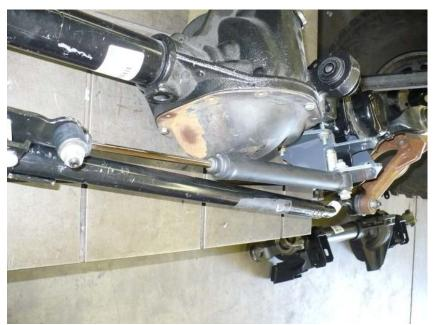
16. Reattach the track bar using the factory nut and bolt, it helps to have someone turn the steering wheel to align the track bar to the hole in the bracket. Torque the factory track bar bolts to 125 ft-lbs (170 N-m). Remember to tighten the track bar frame mount bolt if you loosened it earlier.
