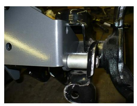
5. Insert the shortest of the 3 spacers where the stock track bar bushing was. Install the 9/16 x 3" bolt in the track bar relocation bracket through the stock track bar mounting hole. Use a flat washer under the bolt head and under the lock nut.
