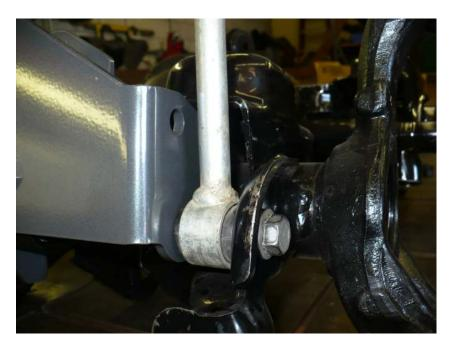
13. Install the steering stabilizer to the track bar relocation bracket. Attach the body end of the steering stabilizer to the track bar relocation bracket using the factory nut and bolt.
