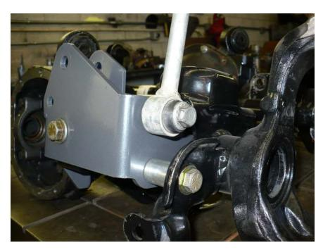
11. Install the driver side anti-sway bar relocation bracket using a 1.5" (38 mm) spacer and ½" x 3" bolt and top-lock nut; use a washer under the bolt-head and nut. Tighten the ½" bolt to 90 ft-lbs (120 N-m), and the sway bar link bolts to 90 ft-lbs (120 N-m).
