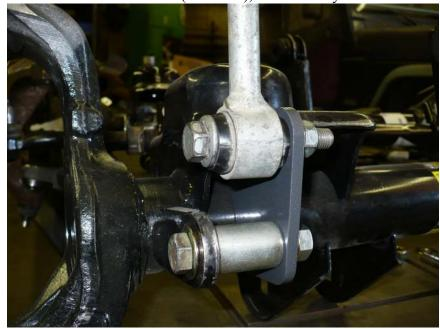
12. If you are not using the anti-sway bar relocation brackets and want to mount the sway bar links in the factory location, install the passenger side anti sway bar link between the track bar bracket and factory sway bar tab as shown below. Attach the driver side anti-sway bar link in the factory location.
