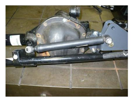
15. Rotate the tie rod clamp forward enough that the steering stabilizer clears the diff cover. Turn the tires all the way to both sides to verify clearance and that the steering stabilizer does not limit the steering angle. When the tie rod clamp is positioned correctly, tighten the clamping bolt.
