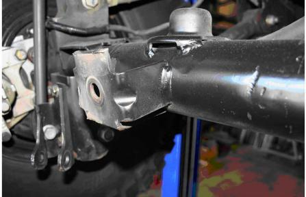
3. Attach the new track bar relocation bracket to the factory bracket as shown with the new 9/16" bolt and lock nut, use a flat washer under the bolt head and lock nut.
