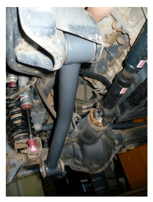
3. Remove the existing lower control arms. If you are just replacing the lower control arms, they can be replaced one at a time with the vehicle sitting on level ground, without removing the tires & wheels or any other suspension part.
