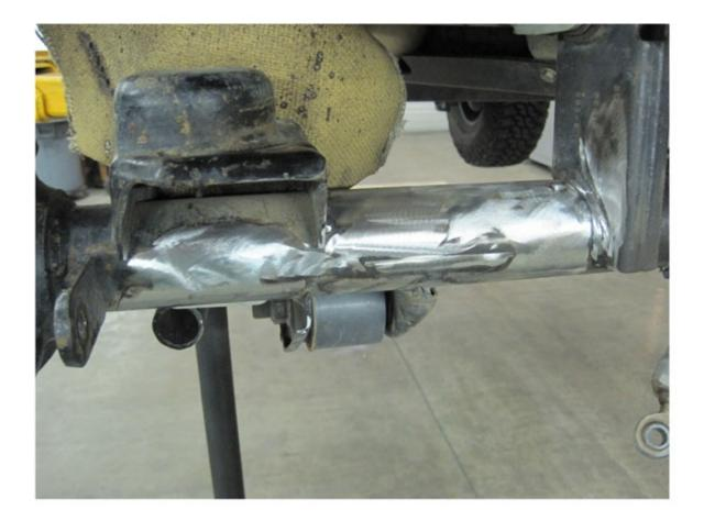
3. Locate the new weld on track bar bracket using a 1 ½" long spacer between the lower side hole of the track bar bracket and the stock sway bar tab. This spacer is not provided, you can also use your stock sway bar link as a spacer.
