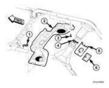
4. Remove the upper bolt to the seat belt turning loop height adjuster.
