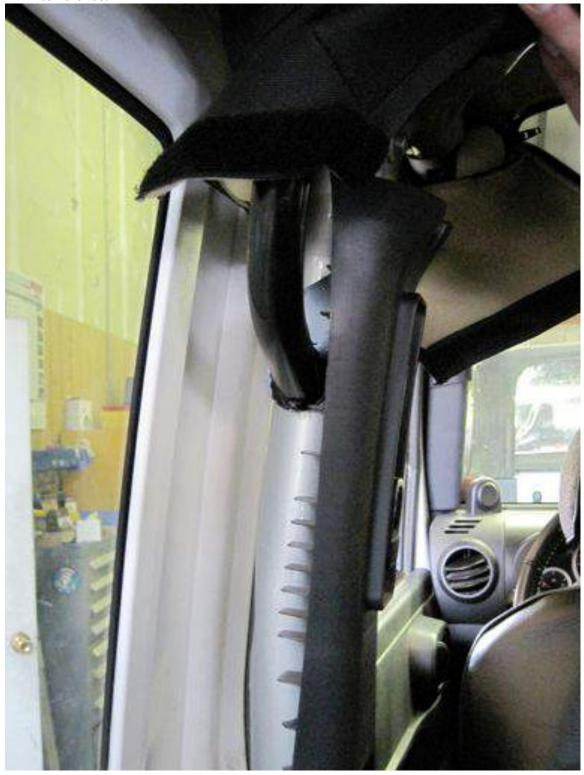
7. Remove the grab handles. Secure the upper grab handle bracket using the speaker pod bolts, do not fully tighten yet. Secure the lower bracket of the grab handle under the seat belt turning loop height adjuster and torque to 30 ft-lbs. Reinstall all trim and padding at this time. Remove the speaker pod bolts and install the speaker pod and tighten the screws to 7 ft-lbs.
