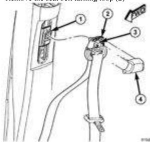
2. Unzip and remove the rollbar padding from around the b-pillar and, using a trim stick C-4755 (interior trim removal tool) or equivalent separate
