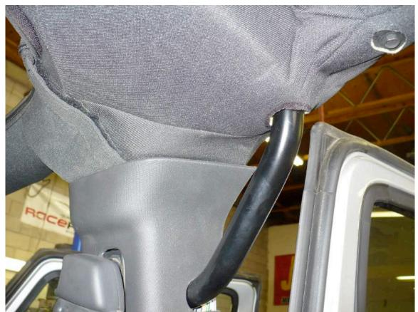
7. Notch the B-pillar trim as shown. A PDF template is provided online, print and cut the template out with scissors. <a href="http://www.synergymfg.com/instructions/JK-Grab-Handle-Pattern.pdf">http://www.synergymfg.com/instructions/JK-Grab-Handle-Pattern.pdf</a>
