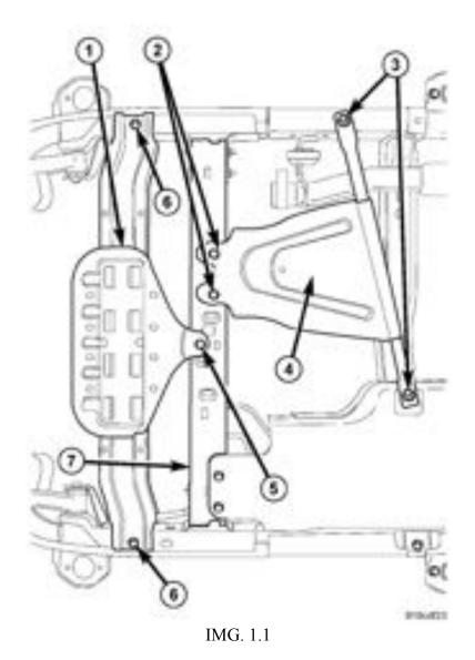
2. After removing the skidplates, remove the 3 nuts securing the transmission mount to the transmission cross member. Use a 16mm socket for removal.
