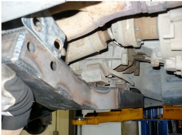
8. Next, go ahead and lower the weight of the transmission onto the cross member and reposition the jack under the cross member itself. Place a jack under the cross member and lift it just before the vehicle itself starts to lift. This step is done to optimize ground clearance as there is significant play in the factory mounting holes on the frame.
