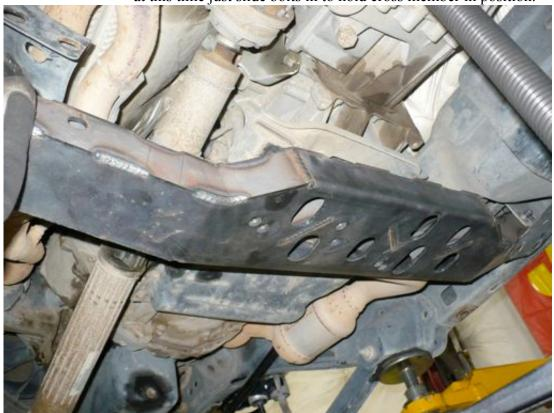
• Align the transmission mount with the appropriate holes in the cross member and install the bolts in the passenger side frame mount labeled #1 in Img 4.1 above. Again, do not install nuts at this time just slide bolts in to hold cross member in position
