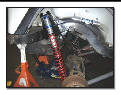
This kit is designed to use most twin tube or monotube shock absorbers. Shocks we recommend are: Fox 2.0 coilovers, air shocks, or smooth body shocks; Sway-a-Way 2.0 coilovers or air shocks; Edelbrock Xtreme IAS shocks, or our Poly Performance BBCS shocks.
