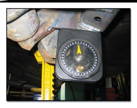
mount can be rotated up or down depending on the placement of the upper mount and shock alignment.
