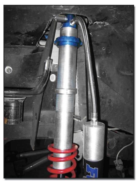
**Figure 4: Correct Shock Mount Position**
