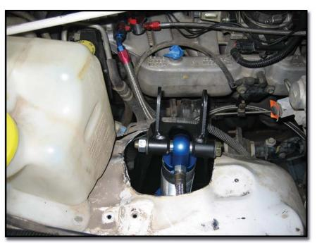
Figure 3: Fender cut for shock mount
