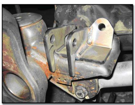
**Figure 5: Lower Shock Mount Position**
