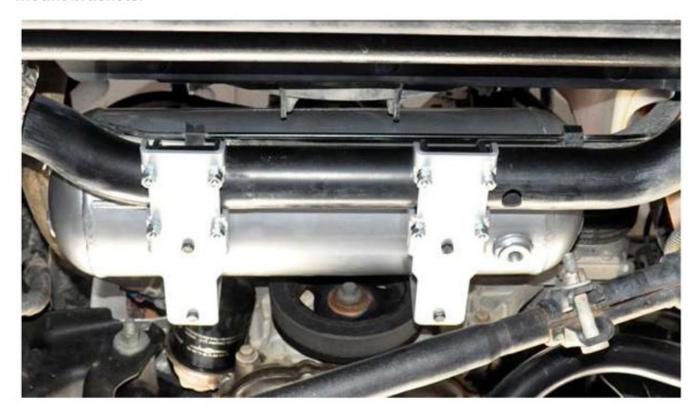
8. Install the next 8 nuts and tighten them as jam nuts.
