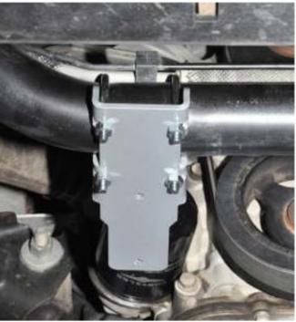
2. Place the tank mount bracket into position and firmly hand tighten all four nuts on the passenger side.
