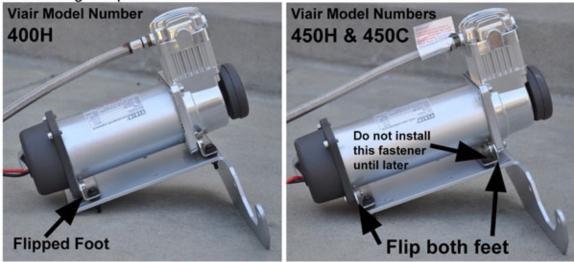
400H - The foot flip procedure for the 400H is complete at this time. Proceed with the standard compressor mount bracket instructions at this time.
