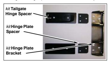
a. On inner two holes of hinge, Install using *kit* **bolts** (8mm-1.25 x 50mm) with **taper washers** (8mm). Do not tighten at this time.
