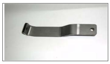
a. On underside of body top mount plate, place bracket end on upper outer long hinge bolt shown. Secure with *kit* **nut** (8mm flange)
