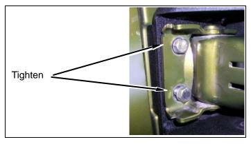
d. Tighten Landing block position so hook area of block just has enough clearance for landing bar of rack, block is slotted for this adjustment. Adjust rack latch hoop and tighten jam nut, this will allow the latch to properly cam-lock itself when in closed position.
