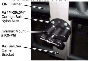
t. Install the fuel can on the carrier by inserting the center of the fuel can on the *Rotopax* mount and twist the wing nut until the fuel can is secure.
