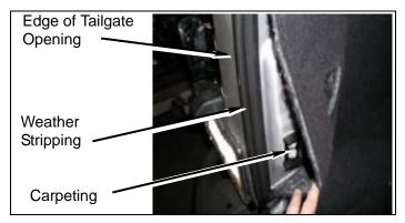
b. Find the center of the door chanel and measure from inner lower corner of body up 3 7/8" for first hole location and 10 7/8" for second hole location center punch and drill 7/16" hole on each as shown. (Note: Be sure to measure against flat sheet metal surface and not on top of body seam puddy. All JK's may need some minor adjustments made to these holes once bracket is set in place; due to variances in body panel positioning.)
