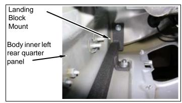
c. Insert kit landing block mount bracket under left rear of body and align holes in bracket to holes drilled. Make sure bracket is snug to inner body corner. Install kit bolts (5/16" x 3/4") and washers into bracket and snug but do not tighten.
