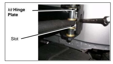
c. Now open carrier rack and tailgate to tighten inner hinge plate bolts.
