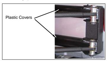
f. Install on the back side of upper and lower hinge plate using *kit* **nut** (8mm flange) and tighten (exclude upper outer longer bolt for next step.)
