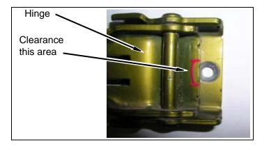
a. Mark and grind out area shown on factory tailgate hinges to allow clearance for *kit* **bolt** (8mm & tapered washer) and wrench during install.
