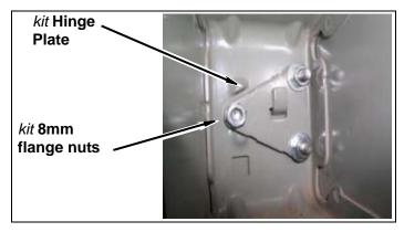
14. Install kit hinge plate upper support bracket
