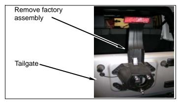
b. Remove grommet and wire harness from tailgate.
