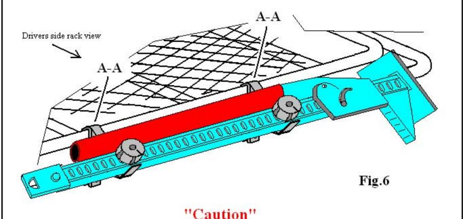
"Use Caution when installing or removing High Lift Jack from brackets as they may slip from your hand causing serious injury or damage to your vehicle."
