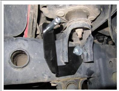
Fit the sway bar disconnect park brackets to the chassis rails.
