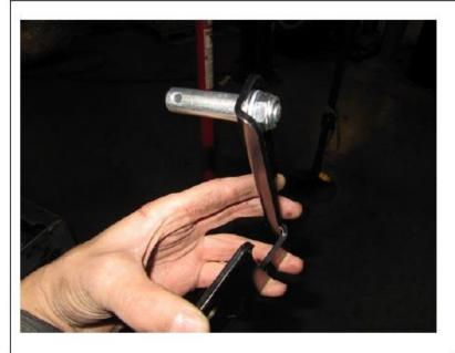
For all models other than Rubicon, a sway bar disconnect system is provided in the kit.
