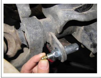
Fit greasable sway bar link pin and nut to axle bracket. Fit the grease nipple and tighten with spanner.
