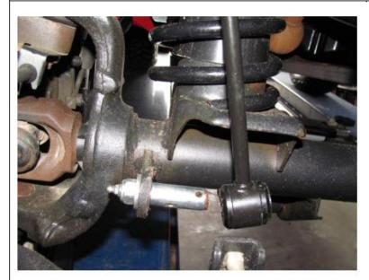
Install new sway bar linkage as shown.
