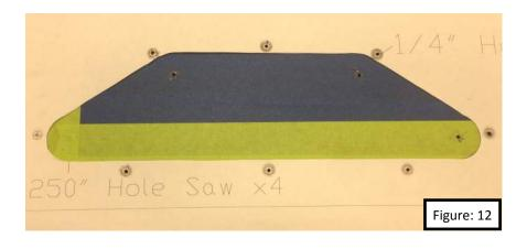
17. Trace the shape of the center hood vent hole that will be cut into the hood. Figure: 13
