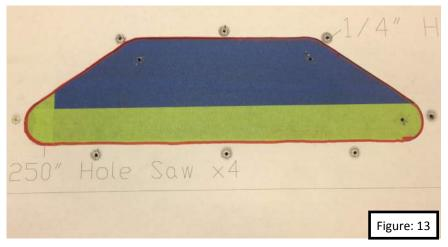
18. Open up the four (4) holes located in the interior of the vent. Use the 1-1/4" hole saw for this operation. Figure: 14
