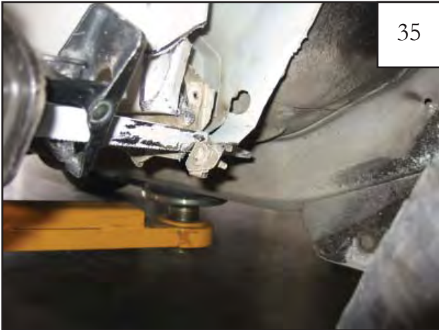
Use a saws all to cut off remaining sheet metal and bolt.
