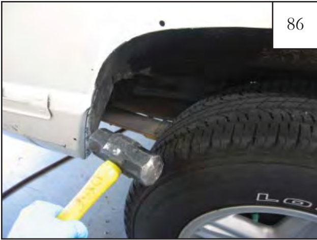
Use a small sledge hammer to flatten out sheet metal tabs. Remove the tire if desired to make hammering easier. Avoid bending or distorting outer sheet metal.
