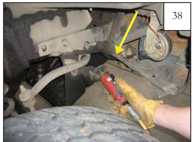
(For 84-96 Model Years Only) Use a cut off saw to trim fender support bracket on the inside front portion of wheel well.
