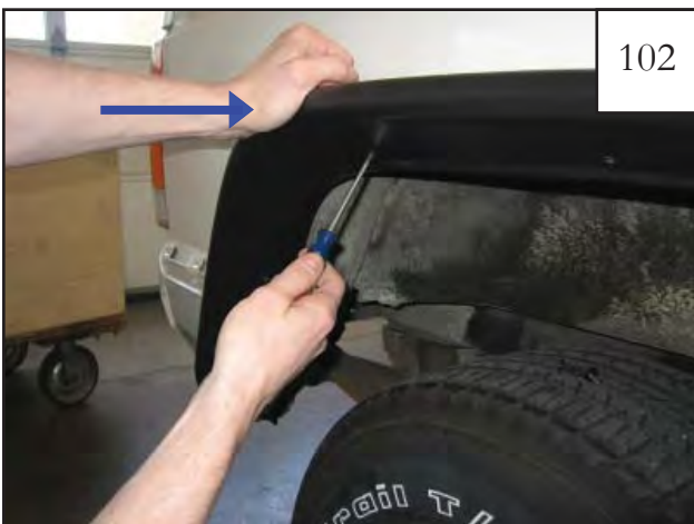
Hold flare in place on fender and start a #8 pan head screw into each hole location and through speed clip on inner structure (6 places). Do not tighten.
