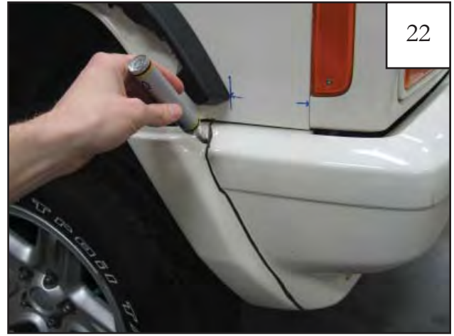
22 (For 97-01 Model Years Only) Use a grease pencil or marker to make a line on the factory front bumper for trimming.
