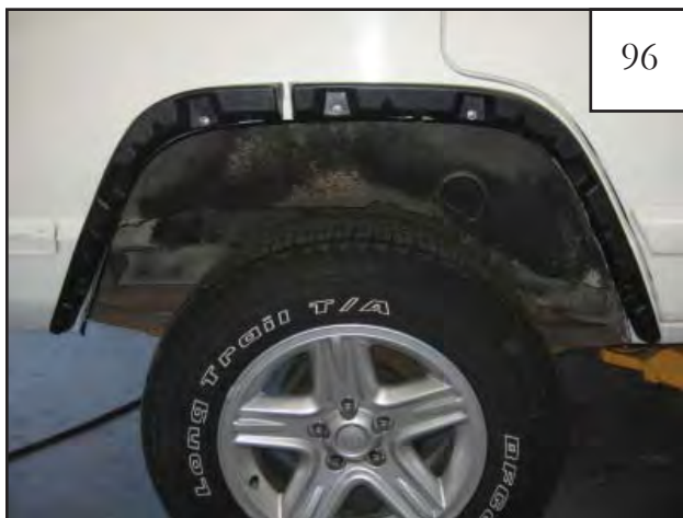
Inner pieces installed.
