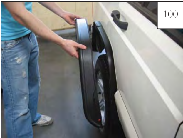
Place the outer flare over the inner pieces and push until snug against the sheet metal.
