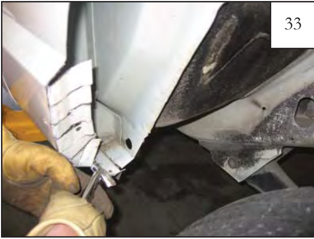
Use pliers to bend back sheet metal tabs.
