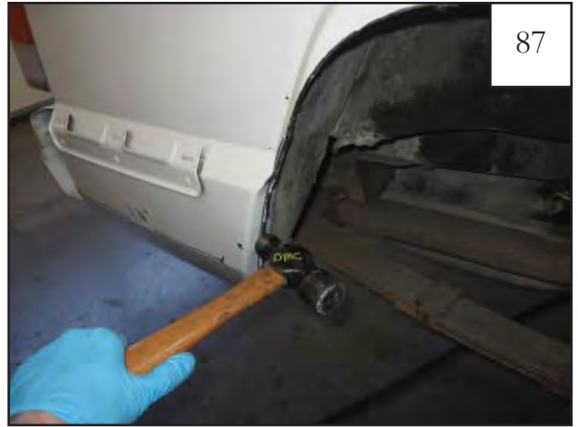
Use a ball peen hammer to further flatten and even out sheet metal.
