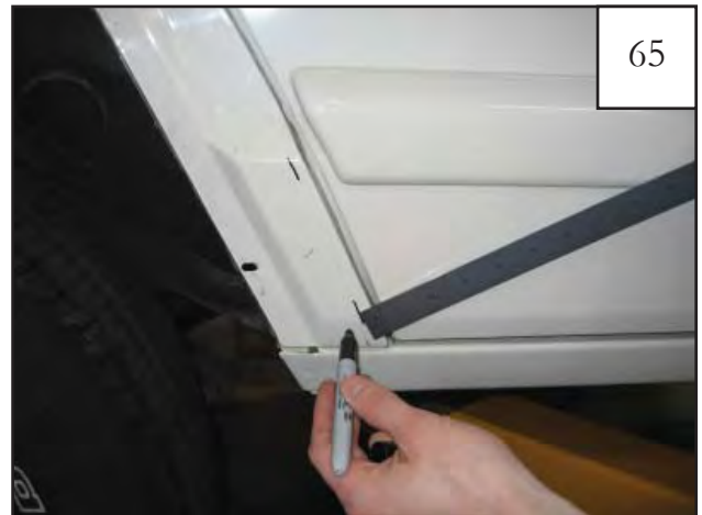
(For 4-Door Vehicles Only) Use a grease pencil or removable marker to make a line parallel with the door seam 3/8 " away from the door seam.
