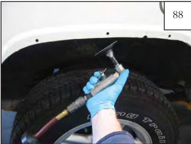
Use an angle grinder to sand and even out trimmed wheel well sheet metal. Use caulking or primer to seal any exposed sheet metal if desired for rust prevention.
