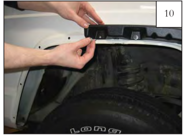
Slide washer onto M5-8 machine screw. Insert a screw/washer assembly through inner flare piece and fender and secure with a flange nut. Only hand tighten at this time.
