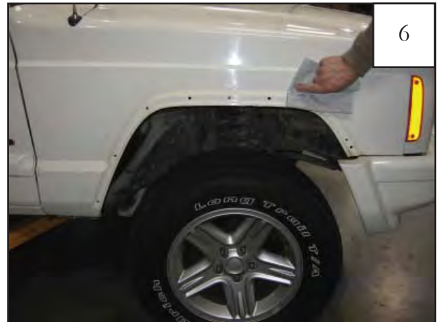
With the factory flares, splash shield, and body side molding removed, thoroughly clean the exposed metal fender with a damp cloth and dry.
