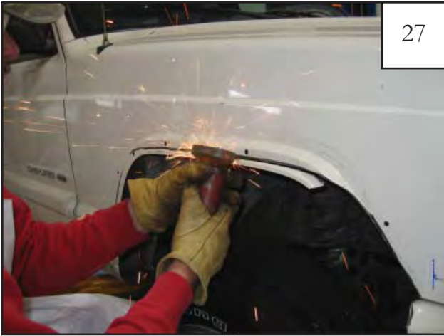
Use a cut off saw to cut the front fender along marked line. Do not cut any sheet metal past where the horizontal lines were marked in step 24. See next photo for fender image after trimming.
