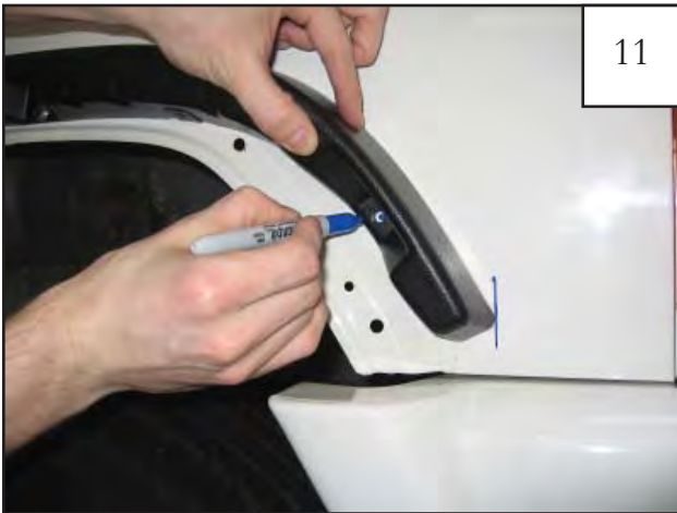
Align outer edge of inner piece P1 (D1 for driver side) with the measuring line made in Step 9. Use a grease pencil or marker to mark the front hole location on the sheet metal.
