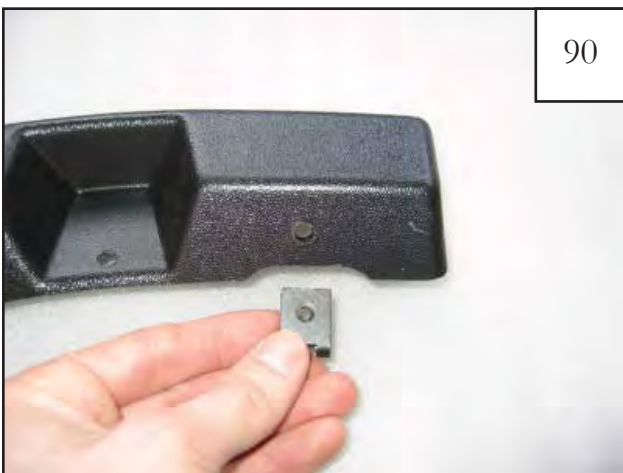
Install a speed clip at each clip location on the inner pieces, centering them on the predrilled holes. (6 locations)
