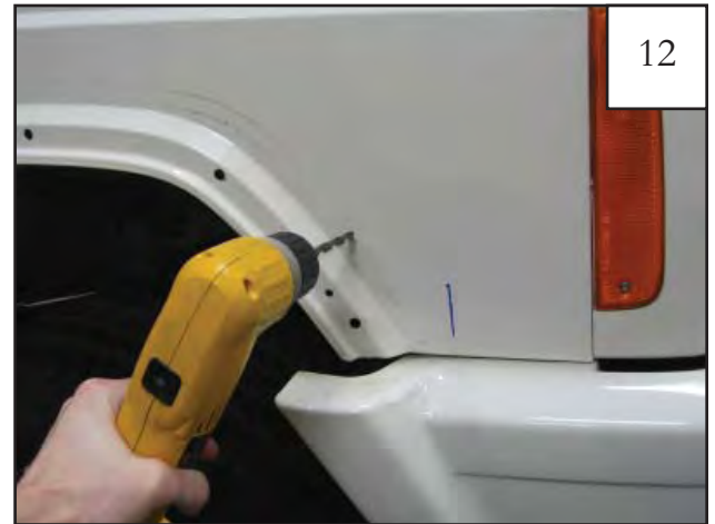
Remove inner piece from front fender. Using a 1/4" drill bit, drill through sheet metal on location marked in previous step. Pre-drill with a smaller drill bit if desired.
