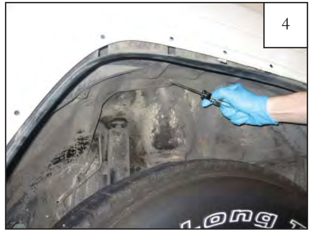
Remove inner splash shield from wheel well using a pry tool or other suitable tool (7 locations). Save splash shield for trimming and reinstallation.
