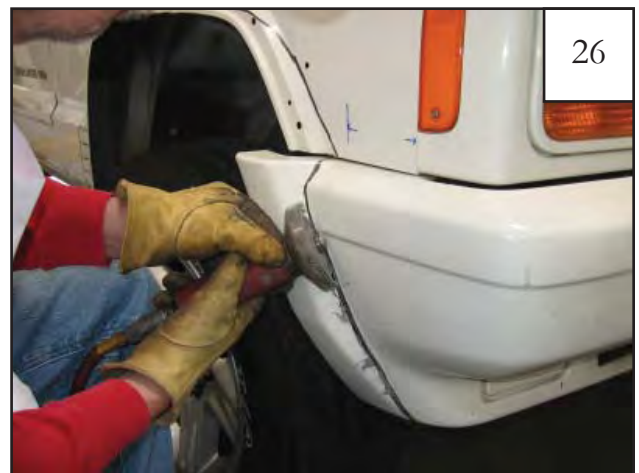
26 (For 97-01 Model Years Only) Use a cut off saw to cut front bumper along marked line.
