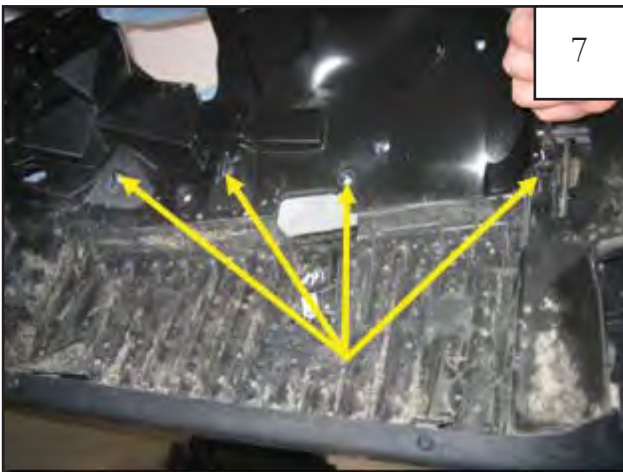
Use a pry tool or flat head screwdriver to remove four plastic fasteners.
