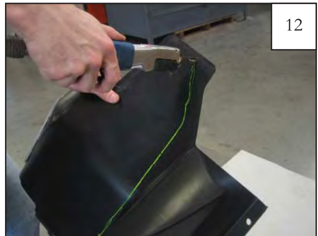
Remove splash shield. Save factory hardware for reinstallation. Using a metal hacksaw, pneumatic hand saw, or other suitable cutting device, trim the splash shield along the marked lines.
