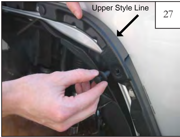
Step 2 While holding the inner piece in place, install a plastic push retainer through holes in both inner pieces. Inner piece should rest along upper style line of sheet metal radius and not below it: see step 22.
