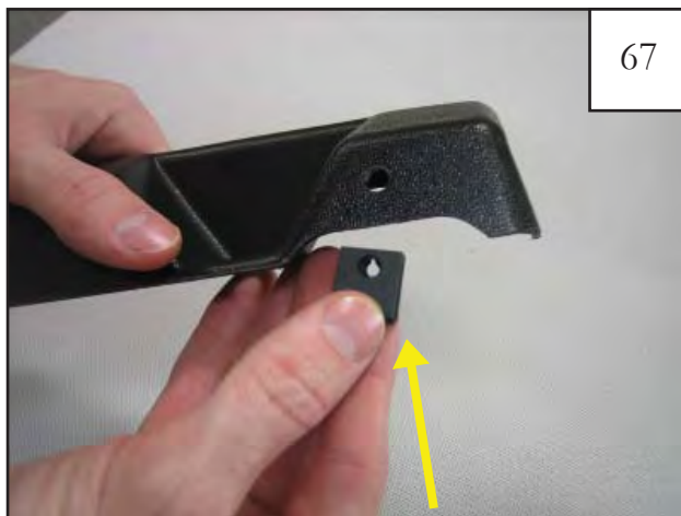
Install a speed clip at each clip location on the inner pieces, centering them on the predrilled holes with threaded portion on inside. (6 locations) NOTE: Clips may slide out of place. Try pinching the metal tightly onto the inner piece with pliers.
