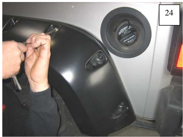
Remove three rearmost screws installed in Step 20.
