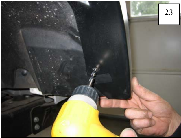
Holding the splash shield firmly, drill through rearmost hole in flare and through the splash shield using a 5/16" bit.
