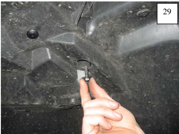
Reinstall the factory bolt in hole in splash shield as shown.
