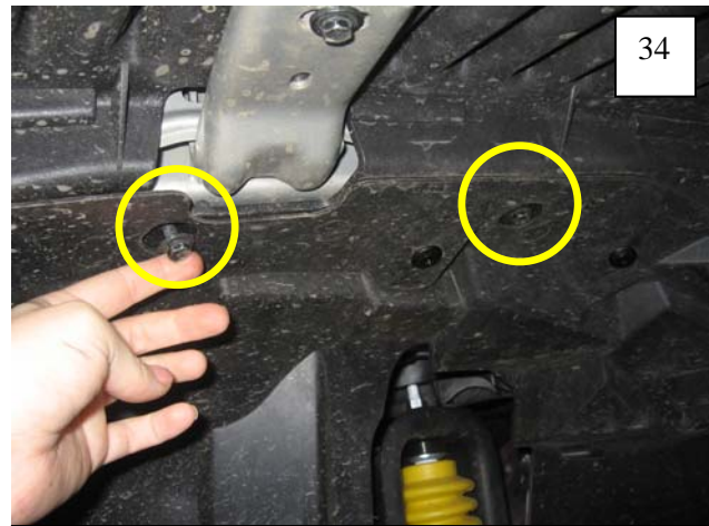
Reinstall two factory bolts as shown.
