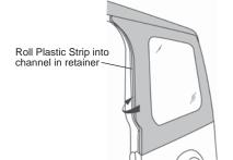
Locate the two plastic strips sewn to the sides of the top, above each door. Slip the strips into the channel in the Door Surround above the door opening. It is easiest to insert the front plastic strip into the channel first.
