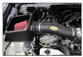
14. Install the Airaid Premium Filter (#1) onto the Filter Adapter.
