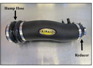
10. Slide the Hump Hose (#6), and two #68 Hose Clamps (#21), onto the Intake Tube as shown. Slide the Reducing Coupler (#7) and the #48 (#19) and #64 Clamps (#20) on the other end of the Intake Tube. Leave the Clamps loose for now.
