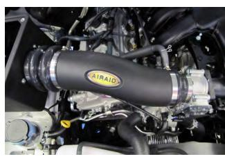
11. Install the Airaid Intake Tube onto the Cold Air Box and the throttle body, align and tighten all four of the Clamps. Reconnect the Mass Air Flow sensor.
