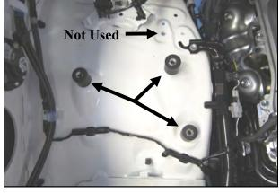
**5.** Install the three M8 CAB Mounts (#13), hand tight, into the weld nuts on the inner fender as shown. Note: One of the original air box mounting holes is not reused.
