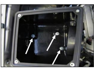
7. Mount the Cold Air Box onto the CAB Mounts using the three 8mm Bolts (#14) and 5/16 Flat Washers (#15).
