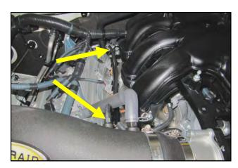
12. Connect the factory crank case breather line to the 3/8 Barbed Fitting on the Intake Tube and replace the OEM vacuum line on the fuel pressure regulator with the supplied 17" 1/8" line. Connect the 1/8" line to the second Fitting on the Intake tube.
