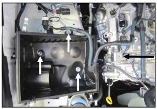
**4.** Pry the wire harness anchor from the airbox. Remove the three anchor bolts in the lower half of the airbox and remove it from the vehicle. Remove the factory intake tube bracket from the valve cover. It will not be reused.
