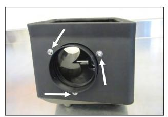
7. Mount the Filter Adapter (#5) to the Cold Air Box, as shown, using three  $1/4-20 \times 1/2$ " Button head Bolts (#16) and 1/4" Flat Washers (#17).
