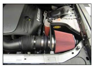
**16.** Install the Weatherstrip (#8) onto the top edge of the Panels with the contour rolling away from the Filter area. Complete the installation by attaching the Airaid Premium Filter (#1) to the Filter Adapter.
