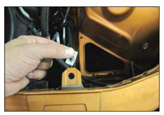
**3.** Carefully remove the speed clip from the core support tab and set it aside. It will not be reused.
