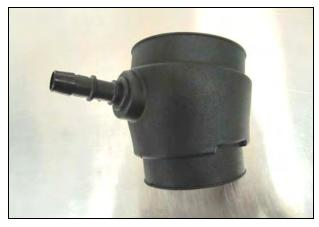
11. For 3.6L V6 Pentastar equipped vehicles: Locate the V6 Airaid Intake Tube marked KIT-210-6T and insert the smaller, 5/8" Grommet (#24) into the side. Complete the V6 Tube assembly by inserting the smaller, 5/8" Barbed fitting (#27) into the Grommet.
