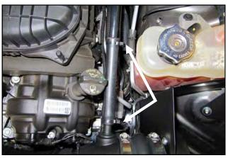
**16.** For **3.6L V6 Pentastar equipped vehicles:** Install the Smaller, 5/8" hose (#11) onto the Barbed Fitting and factory hard line. Snap a Speed Clamp (21) on each end of the hose to secure it in place.
