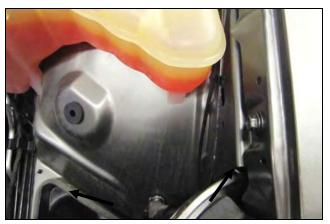
**8.** Remove and save the factory 6mm fender bolt. It too will be reused in step **9**.
