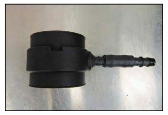
**12. For 5.7L V8 HEMI equipped vehicles:** Locate the V8 Airaid Intake Tube marked KIT-210-8T and insert the larger, 3/4" Grommet (#23) and one of the larger, 3/4" Barbed fittings (#25) into the side. Complete the V8 Tube assembly by installing the 2 1/2",
