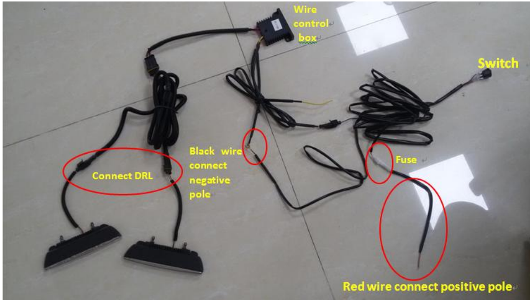
(Complete Wiring Set up)
