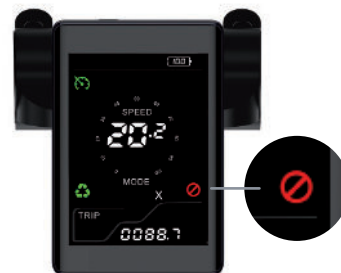
The error code is active, the value will appear in section A.
