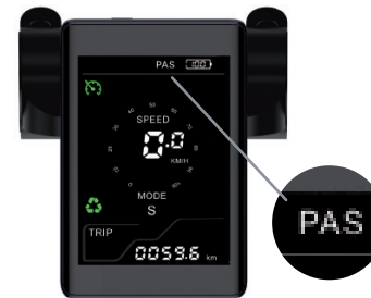
The scooter is in assisted start mode, which means you need to pick up some speed at the start to activate the throttle.
