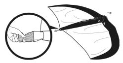
Visually check the bladder for leaks. If the visual inspection has not produced any result, partial areas can be checked with a sponge moistened with water.
