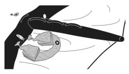
Fold the bladder and use the lines to carefully pull it into the tube. Close the ends of the tube and the zipper.
