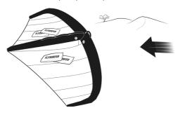
The wing can also be attached to an object with the arm leash to secure it. Keep the leash short to prevent the wing from bouncing on the ground!
