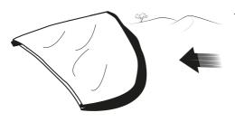
To reduce the pack size, a third of the strut can be folded towards the leading edge beforehand. Avoid kinking the windows.
