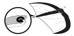
**1** Use the special tool (key) to screw the valves back into the leading edge and strut.
