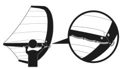
If you move your hand towards the leading edge, you reduce the pressure on the arm. If you bend the arm strongly to pull the wing towards the body, the wing loses power.
