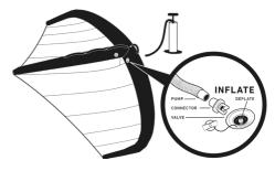
Finally, the wing should be inflated for at least two hours according to PSI information.
