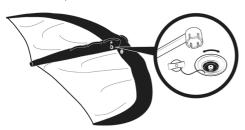
Open the end of the strut and pull the bladder out through this opening.
