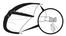
Use the special tool (key) to screw the valve out of the body of the Leading Edge. Loosen the hook-and-loop fastener on the valve connection and press it into the tube.
