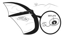
2 Before folding the wing, push most of the air out of the bladder. Place both wingtips on top of each other.
