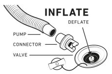
The wing has two free flow valves. Inflate the wing until the strut and leading edge are full. Note the PSI guidelines next to the valve! Close the valve caps before going on the water.
