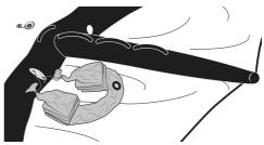
After the bladder is completely extracted from the tube, the lines can be removed and attached to the center of the wing. The lines stay in the body of the leading edge so that the bladder can later be pulled through the tube again.
