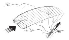
Fold the kite in half along the middle (tip on tip) and make sure that the bridle is inside both halves. Also make sure that there are no bridle lines over the outside skin.
