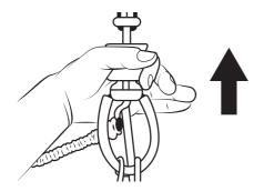
Work your way up the safety endline to the control bar. Wind the loose endline round the bottom of the bar in a figure of 8.
