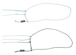
**9** Reconnect the flying lines again, and then repeat the same procedure on the other side. Pull all knots tight and check the bridle carefully.
