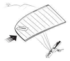
② Open the kite and if necessary, close the deflate valves. Unroll the lines from your bar whilst walking away from the kite.
