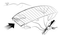
3 Fold the kite in half along the middle (tip on tip) and make sure that the bridle is inside both halves. Also make sure that there are no bridle lines over the outside skin.
