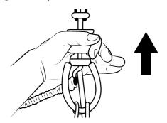
② Work your way up the safety endline to the control bar. Wind the loose endline round the bottom of the bar in a figure of 8.
