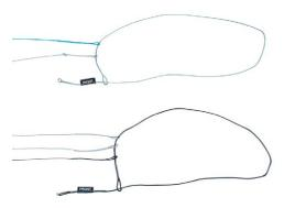
• Reconnect the flying lines again, and then repeat the same procedure on the other side. Pull all knots tight and check the bridle carefully.
