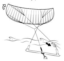
The kite will now spin around. As soon as the leading edge of the kite points up let go of the remaining leader line and put your hand back on the bar. Depower the kite till its back in the sky towards the zenith.
