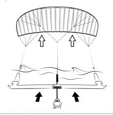
Tip: The reverse launch is the recommended relaunch method when kiting on solid terrain. This minimizes potential damage from abrasion.
