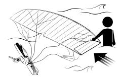
• Lay the tips on top of each other, and then the bar on top and roll up the kite. Be careful with the bridle lines and stow them as best you can within the two halves of the kite when rolling it up. You can open the deflate valves to make rolling it up easier.
