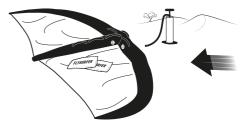
Oconnect the pump to the attachment point in the middle of the leading edge.
