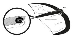
**①** Use the special tool (key) to screw the valves back into the leading edge and strut.
