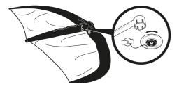
• Open the end of the strut and pull the bladder out through this opening.
