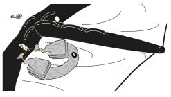
• After the bladder is completely extracted from the tube, the lines can be removed and attached to the center of the wing. The lines stay in the body of the leading edge so that the bladder can later be pulled through the tube again.
