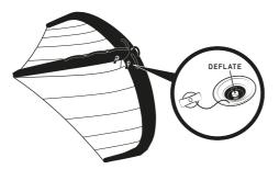
Open the ends of the leading edge and attach a long line to each end of the bladder.
