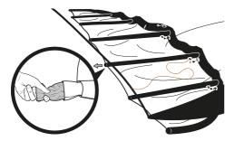
After the bladder is completely out of the strut, the line can be removed and attached to the kite. The line remains in the body of the strut so that the bladder can later be pulled back in.
