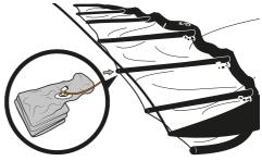
Make sure that the tip of the valve is correctly mounted and cannot slide freely back into the strut!
