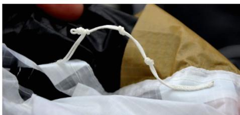
The PMA's are small knotted lines with two settings which are stitched into the aerofoil on the top and bottom. Thereby the aerofoil can be directly adjusted as illustrated below.
