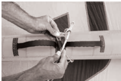
-3- Hold the other side of the harness line and insert it in the lark's head knot
