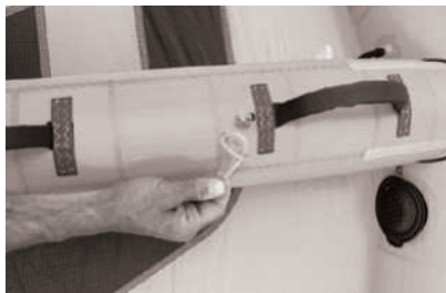
-5- Hold the other side of the harness line and make another lark's head knot.
