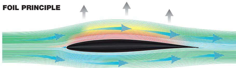
The front and rear wings work as lifting devices, which means they can create a lifting force from the flow of water that travels across them at speed. This is the reason why they are built with a specific sectional profile: The shape of the wings' profile shall not be modified, filled and sanded. Doing so would alter the balance and prevent the correct operation of the foil.
