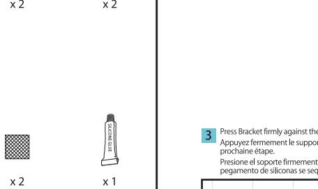
**3** Press Bracket firmly against the wall for 10 seconds. Wait 24 hours for Silicone Glue to cure before proceeding to next step.
