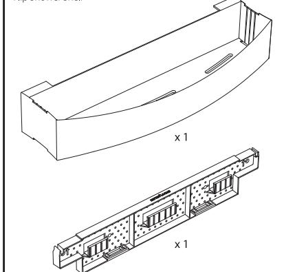
**2** Remove Shelf from Bracket; apply Tape & Silicone to back of Bracket (both required).
